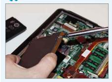
Laptop hard drives are the same size as SSDs, which means you can simply swap one for the other. Remove the battery from the laptop, ground yourself – for example, by touching a radiator – and remove the back of the case. Take out the old hard drive and replace it with the new SSD, then attach the power and SATA connectors and reassemble everything.
