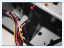
Turn off and unplug your PC, then remove the case. If necessary, unscrew and remove the existing drive. Insert the adapter (with the drive inside) into a spare drive bay and secure it in place. 1 Once that's done, you can attach the power and SATA cables. You're now ready to install an operating system or clone a drive.
