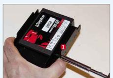
To install an SSD in a desktop PC, you'll need a 2.5in-to-3.5in adapter. Your new drive may come with one but, if it doesn't, you can pick one up for around £7 from the likes of Amazon. Ground yourself to disperse any static electricity, as in Step 1, then insert the SSD into the adapter and screw it in. 1
